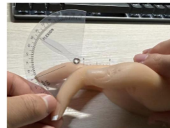
FIGURE 4. The joint angles of the hand model are measured using a professional finger joint protractor
