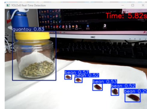
FIGURE 7. Object detection in simulated feeding test
